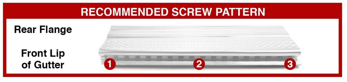
The tab on the left end of each panel installs under the adjoining panel. Use screw holes along the front lip of Waterlock Pro to zip screw the panel - 3 or 4 screws (1, 2 & 3) to the front lip of the gutter. **DIAGRAM 2:** Shows screw holes along the front lip of Waterlock Pro.
